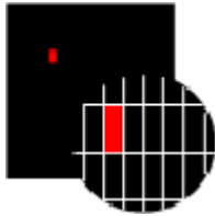
Pixel defect type 3a: Sub-pixel (red, blue, green) constant lightning
