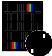
Cluster Pixel defect Type 1: Pixels in a cluster area, constant lightning
